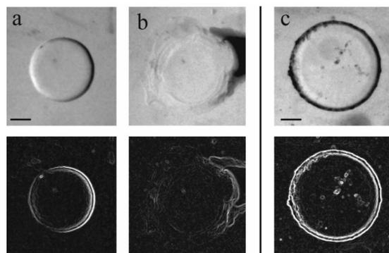
**Figure 1.** Forty-five micrograms per milliliter ALC degrades posts in cream. (a) Initial 310  $\mu\text{m}$  SNAP peptide post in 1  $\times$  PBS,  $t = 0$  h; (b) after 70 h exposure to ALC in cream; (c) control 425  $\mu\text{m}$  SNAP peptide post after 70 h exposure to cream only. Corresponding images directly below a–c are edge-outlined using ImageJ software for better visualization of degraded hydrogels. Scale bars = 100  $\mu\text{m}$ .
