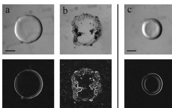
**Figure 2.** Fifteen micrograms per milliliter BoNT/A degrades posts in cream. (a) Initial 425  $\mu\text{m}$  SNAP peptide post in 1  $\times$  PBS,  $t = 0$  h; (b) after 48 h exposure to BoNT/A in cream; (c) 325  $\mu\text{m}$  control post with BoNT/A-insensitive cross-linker after 48 h toxin exposure. Corresponding images directly below a–c are edge-outlined using ImageJ software for better visualization of degraded hydrogels. Scale bars = 150  $\mu\text{m}$ .
